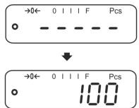
⇒ Remove reference weight. The balance is from now in parts counting mode counting all units on the weighing plate.
